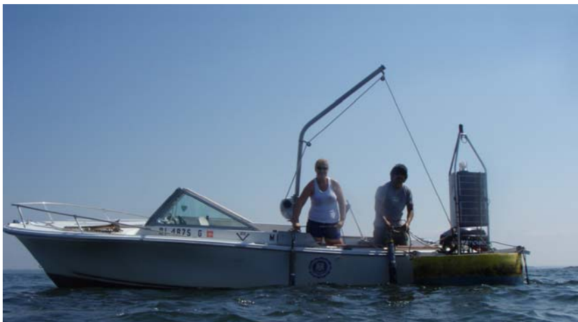
Figure 3a. Surface and bottom sonde deployment at NP buoy.
